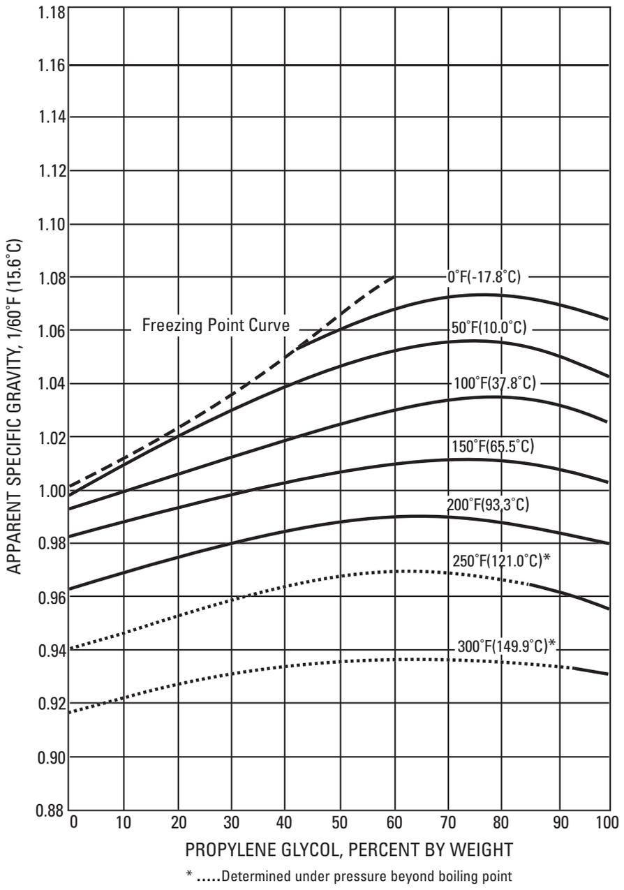
Figure 6 Specific Gravities of Aqueous Propylene Glycol Solutions.
