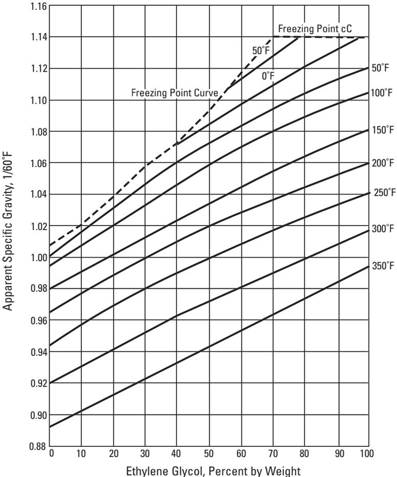
Figure 5 Specific Gravities of Aqueous Ethylene Glycol Solutions.
