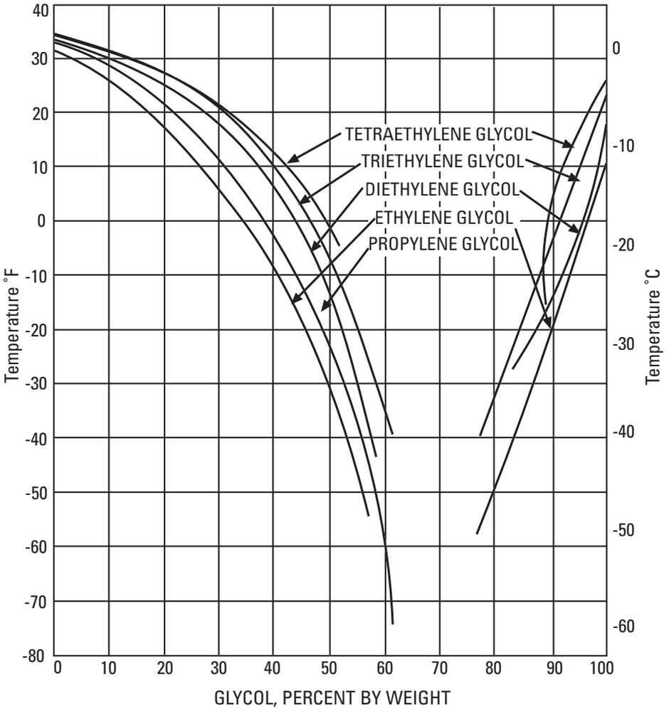
Figure 7 Freezing Points of Aqueous Glycol Solutions.
