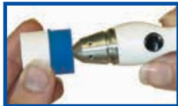
Position the Ocu-Film + applicator on the transducer.
