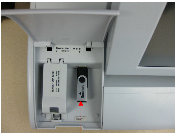
Figure 1. USB Stick plugged into the USB Drive
