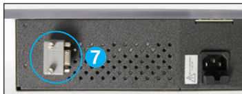
ClearChart 2 w/ serial port at bottom left corner plus Right Angle Serial Adapter 7
