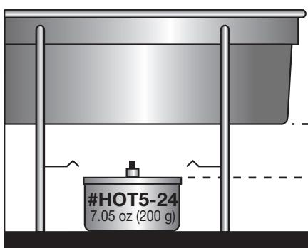
Placement of the Hot 5™ can under the chafer is critically important to get the maximum heat value from the product.
