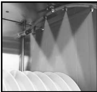
Rainbow Rinse™ produces superior results while significantly reducing water consumption
